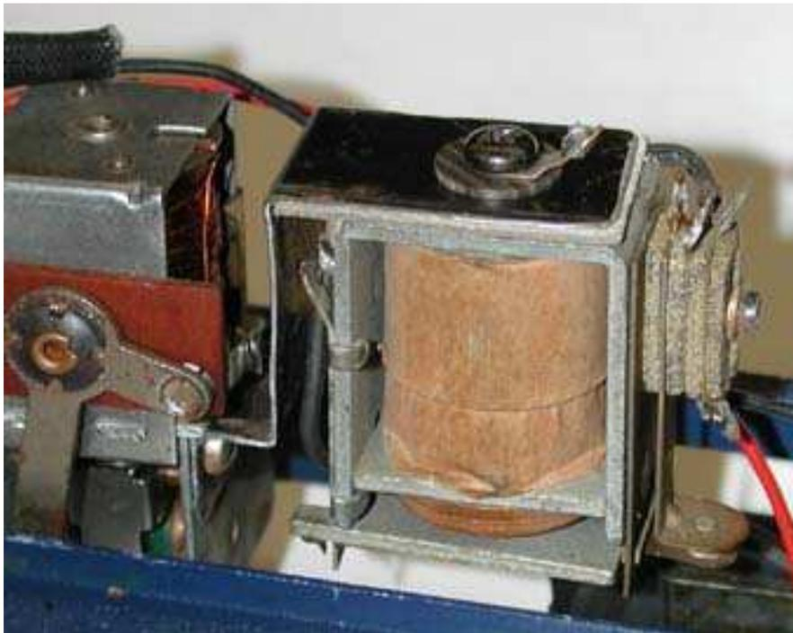
Find the common 'hot' wire that goes to each coil coupler from the slider shoe. Run a wire from the output of the relay contact and solder it to the common wire. Use shrink tubing or electrical tape to prevent shorting to the chassis. You don't have to detach the slider shoe connection. In fact you can still use the remote control track section if the situation demands it.
