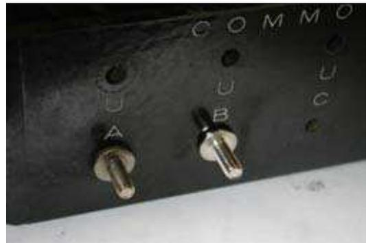
Remove the old post and insert the new one in the hole. Put the loose wire lug over the threaded stud and screw on the nut until it's tight. Make sure no other bare wires are touching the end. Replacing one of the 'U' posts is easier since it's on the top row and there are no loose wires, just the solid buss bar.
