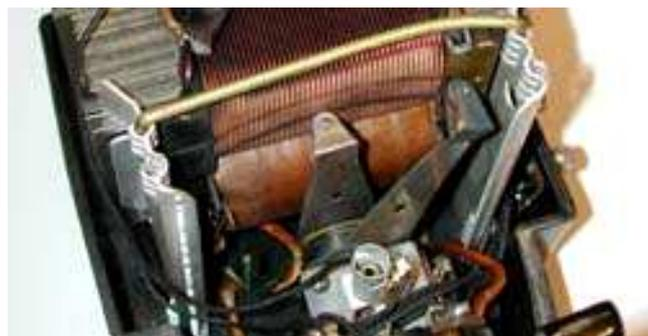
It's usually the "A" or "D" since they are the most utilized. There are two ways to replace rollers; the easy way and the hard way. The hard way entails removal of the short contact arm assembly for the "A" or "D" rollers and the easy way is to install the new rollers in place. Installing the rollers in place means you have to remove the remains of the old rollers and the rivets.
