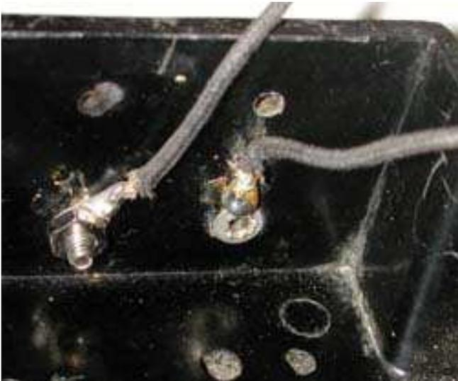
(Note: I usually remove the bottom mounting plate screws that hold the front core aluminum mounting bracket so I can slip the core mounting bracket out of the way (you'll need more room for the bottom posts) when tightening the nuts for the replacement binding posts. Place a small block of wood under the core to hold it in position while working on the posts).
