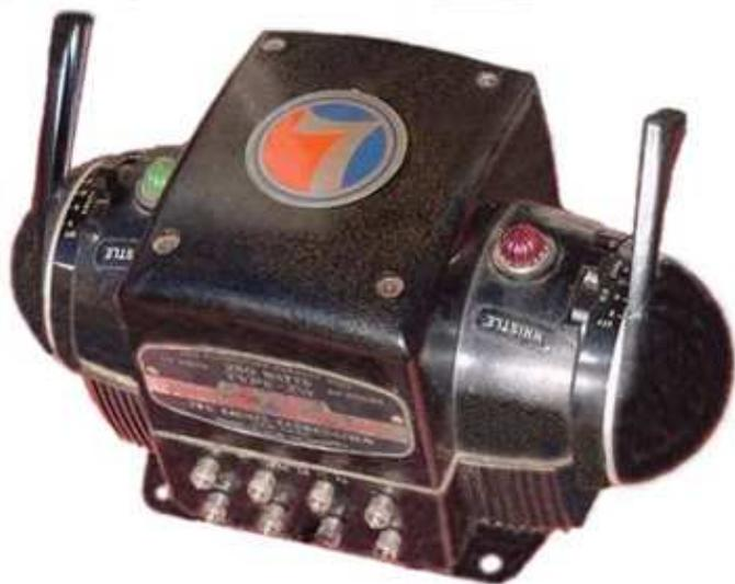
The February Tech Tip addressed how to replace the ZW power cord. This month we will show you how to replace the carbon rollers (four each) and loose or missing binding posts (eight each). Fortunately there are third party replacement parts to rectify both of these common ZW repair problems.
